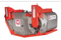
The destemming-chamber isolates the action of the rotor, avoiding it from throwing and then crushing the residuals along the sorting chain, disposing the stalks, stems and leaves quickly. The helicoidal rotor is equipped with techno-polymer moulded
