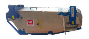
The destemming-chamber isolates the action of the rotor, avoiding it from throwing and then crushing the residuals along the sorting chain, disposing the stalks, stems and leaves quickly.
