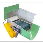
Upper receiving conveyor belt kit, right and left, to direct the harvested product into the destemmers. Made up of a stainless steel frame, 2 rubber rollers, PVC conveyor belt, gearbox and hydraulic motor.
